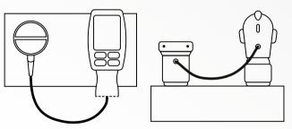
Figure 3: Correct arrangement of transmitter and receiver unit
