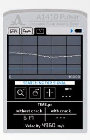
Figure 42: Device ready for crack measurements
