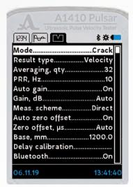
Figure 37: Choosing Crack Sizing mode
