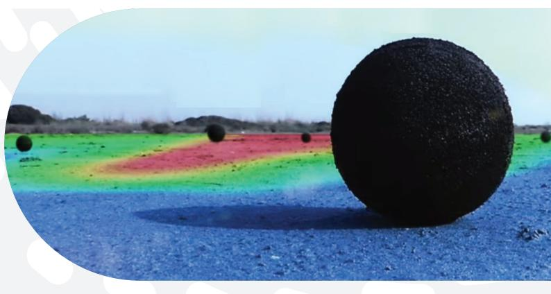
NulSYballs allows fast and remote investigation, monitoring and mapping of hostile and/or accessconstrained areas.
