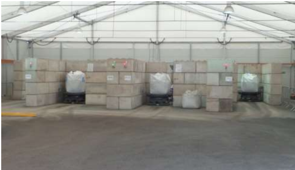
Fig. 8 Photograph of concrete shielding units housing high resolution gamma spectrometry systems for assay of bulk bags
